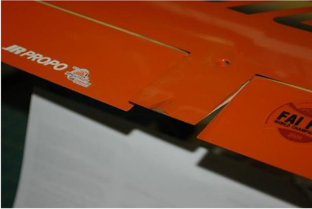
*Here is the trailing edge of a molded, composite structured wing. This shows the “launch-mode” of the model, with flaps partially deflected to increase lift on launch. Ailerons should match this angle as well for best performance.*
